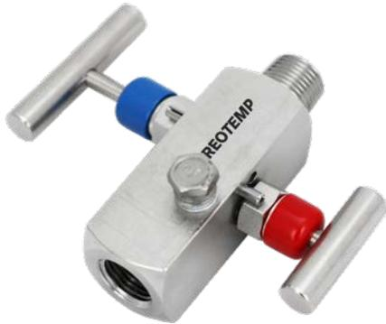
Reotemp's 2-Valve Block & Bleed allows users more options to control their venting. The secondary valve bleeds process through 1/4" FNPT port giving the user the ability to vent to atmosphere or capture the process by directly piping to the valve body.
