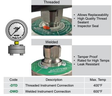
Assembly Notes: Welded connection recommended for pressure exceeding 1,500 psi for purposes of leak prevention.
